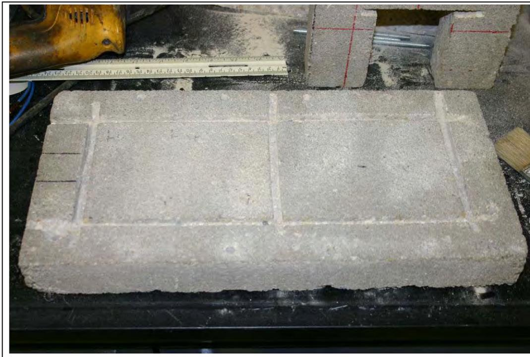
Figure C-3. Floor section with grooves for anodes.
