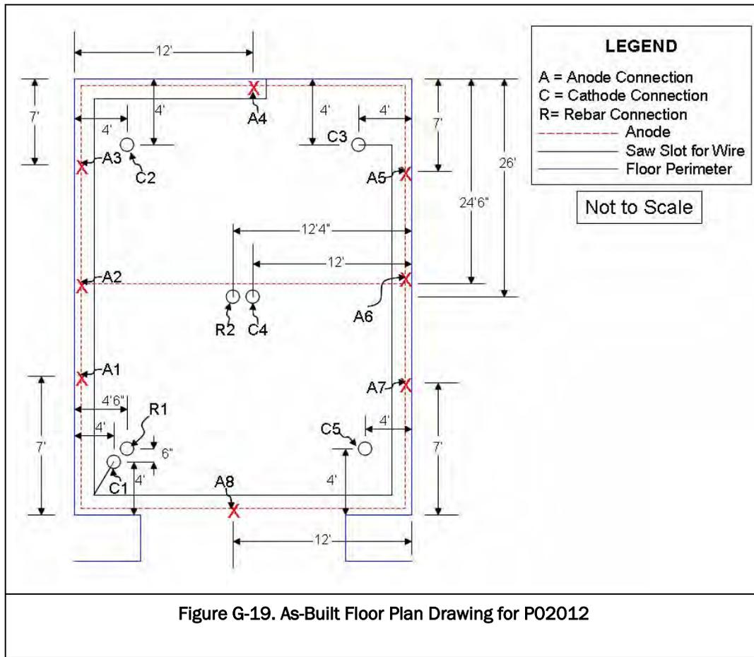
Figure G-19. As-Built Floor Plan Drawing for P02012
