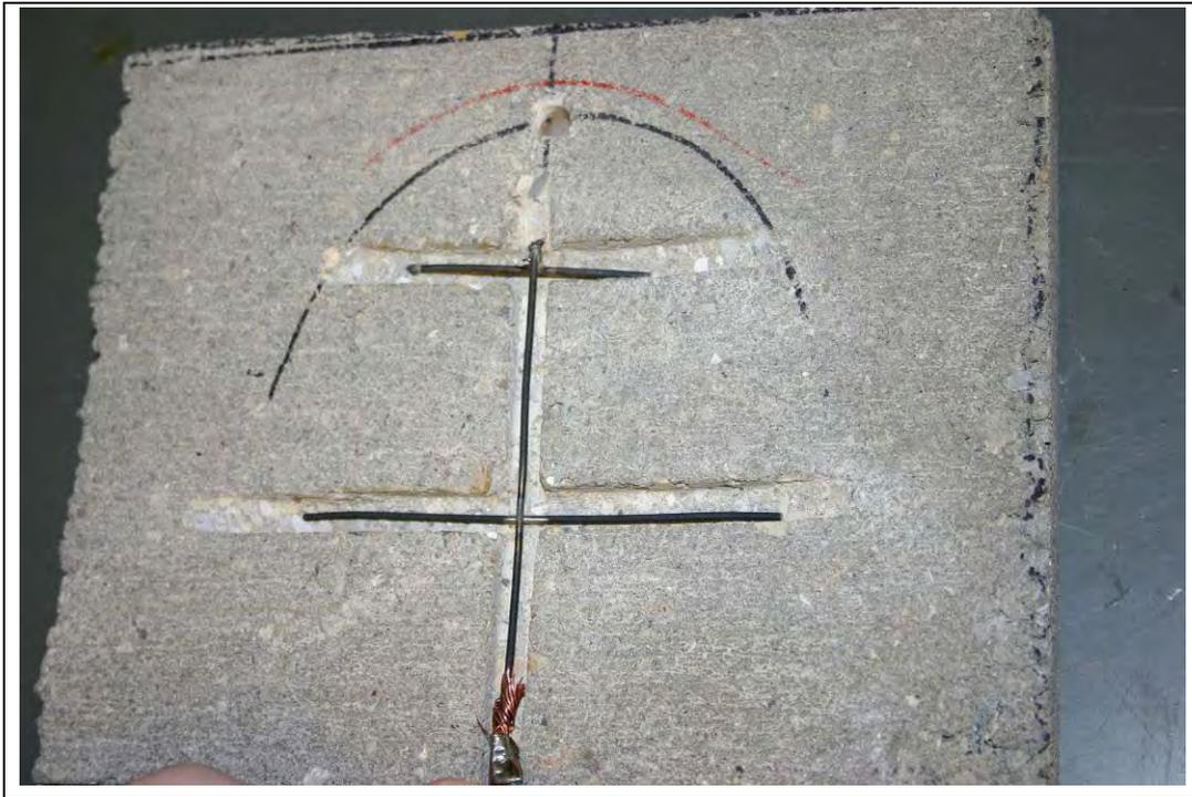
Figure C-4. Rear wall section with anodes in grooves.
