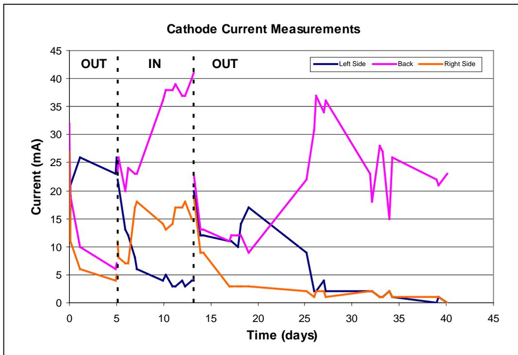
Figure C-16. Cathode currents when cathodes are placed inside (IN) and outside (OUT) ring ground.
