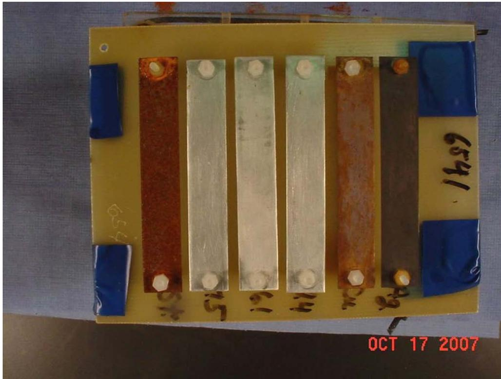
Figure 3.6. Test samples after 3 months exposure outdoors, June – August 2007.
