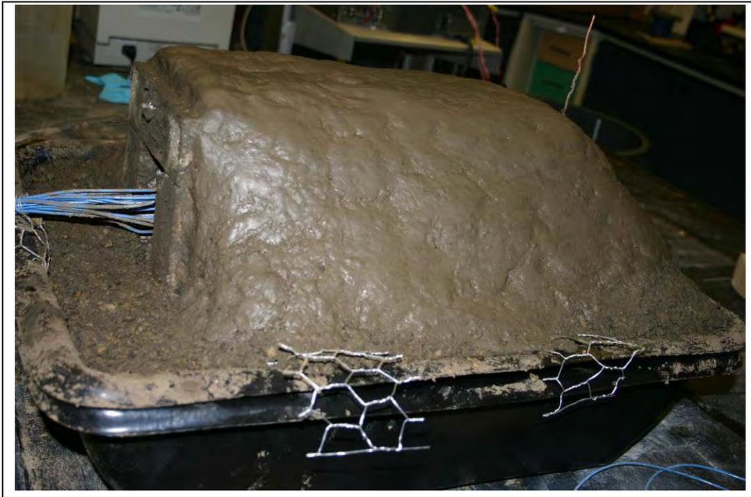
Figure C-10. ECM model with model lightning rod (pulse current injection point) at rear.
