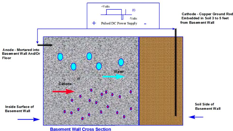
Figure 2.1. Schematic diagram of the EOP system.
