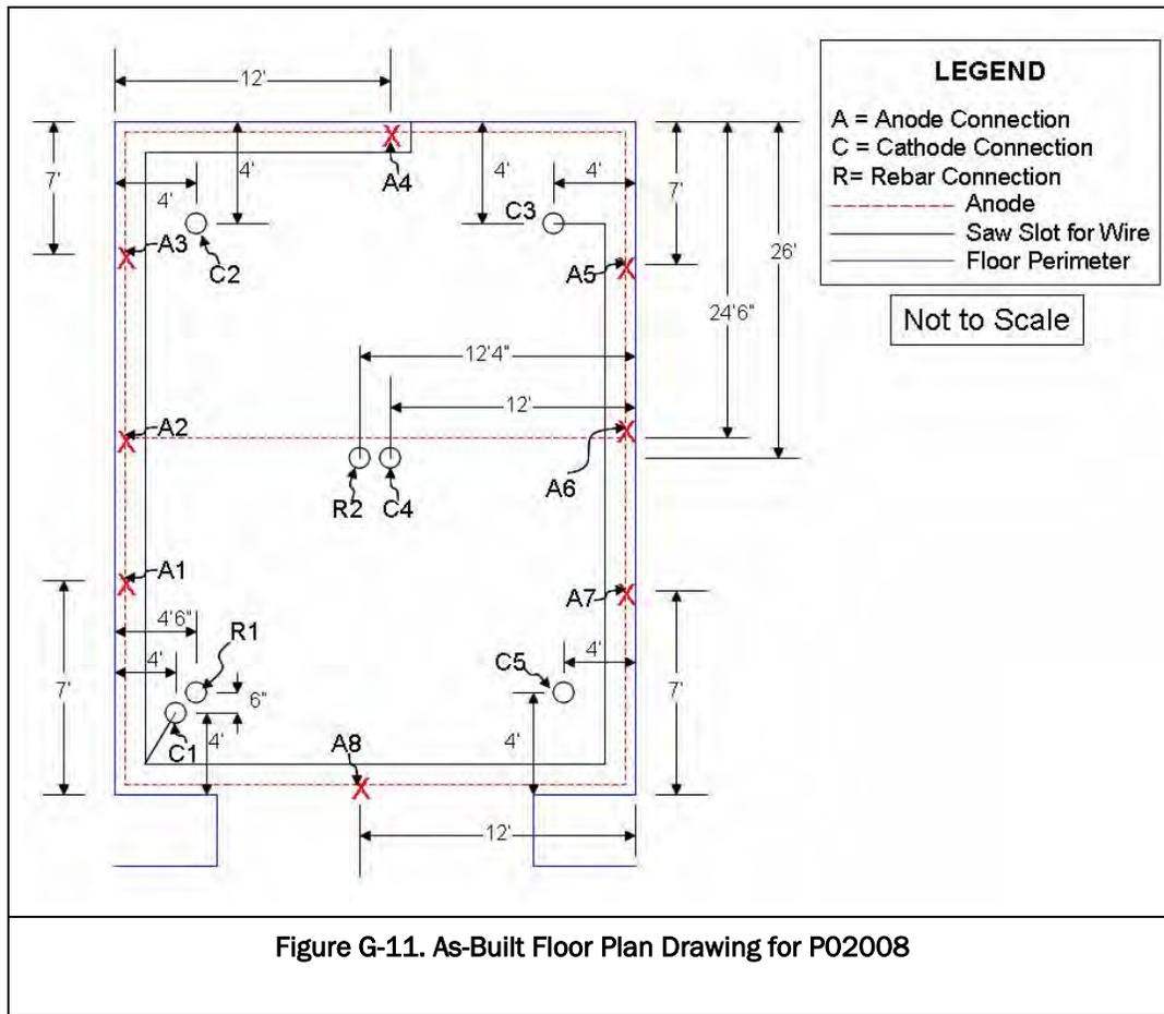
Figure G-11. As-Built Floor Plan Drawing for P02008
