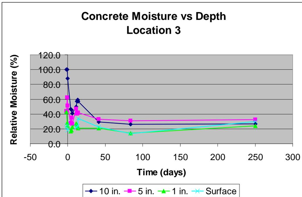
Figure 3.4. Plot of concrete moisture over time at location 3 (Figure E-42).
