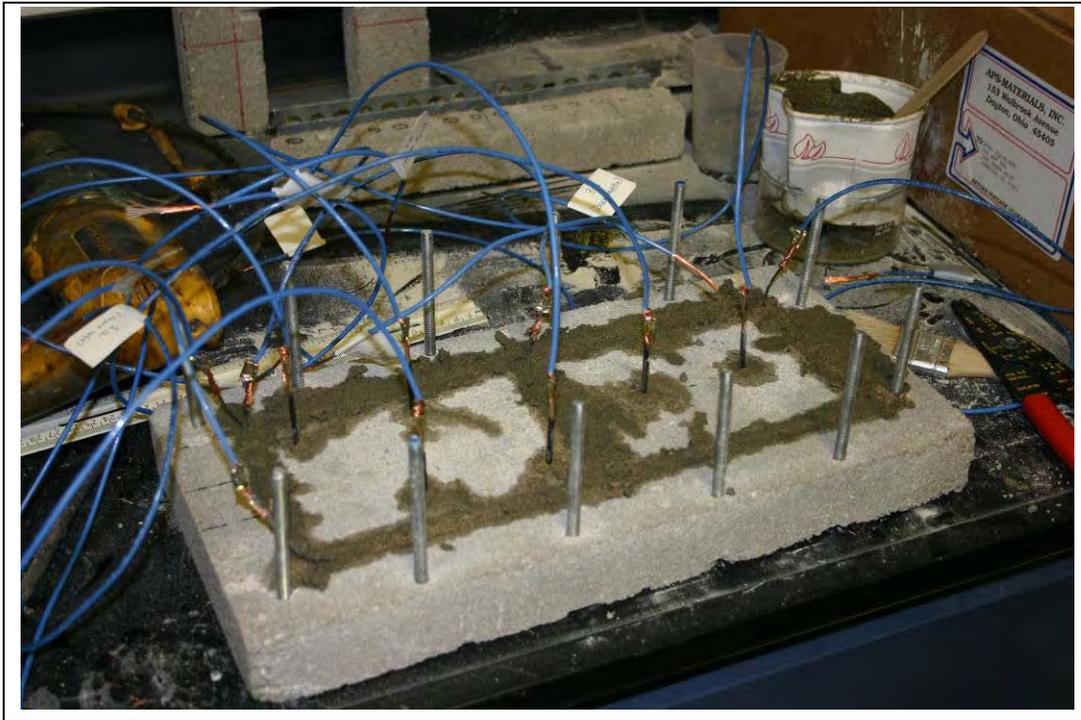
Figure C-6. Floor section with grouted anodes and moisture (Protimeter) probes.
