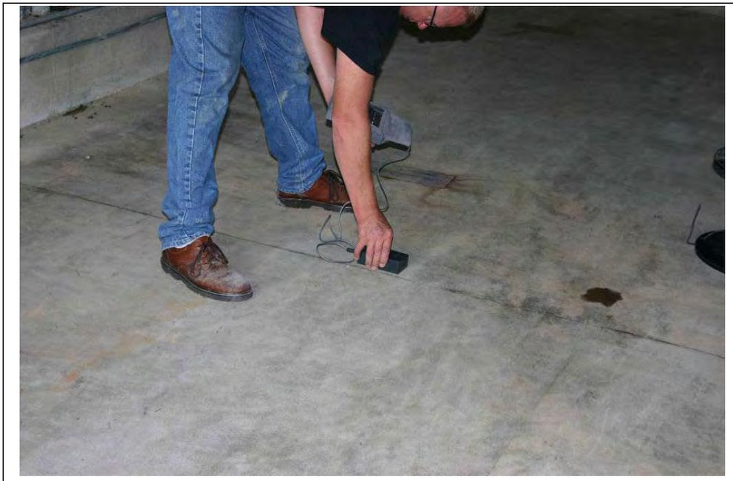
Figure E-1. Locating reinforcing bars in concrete.
