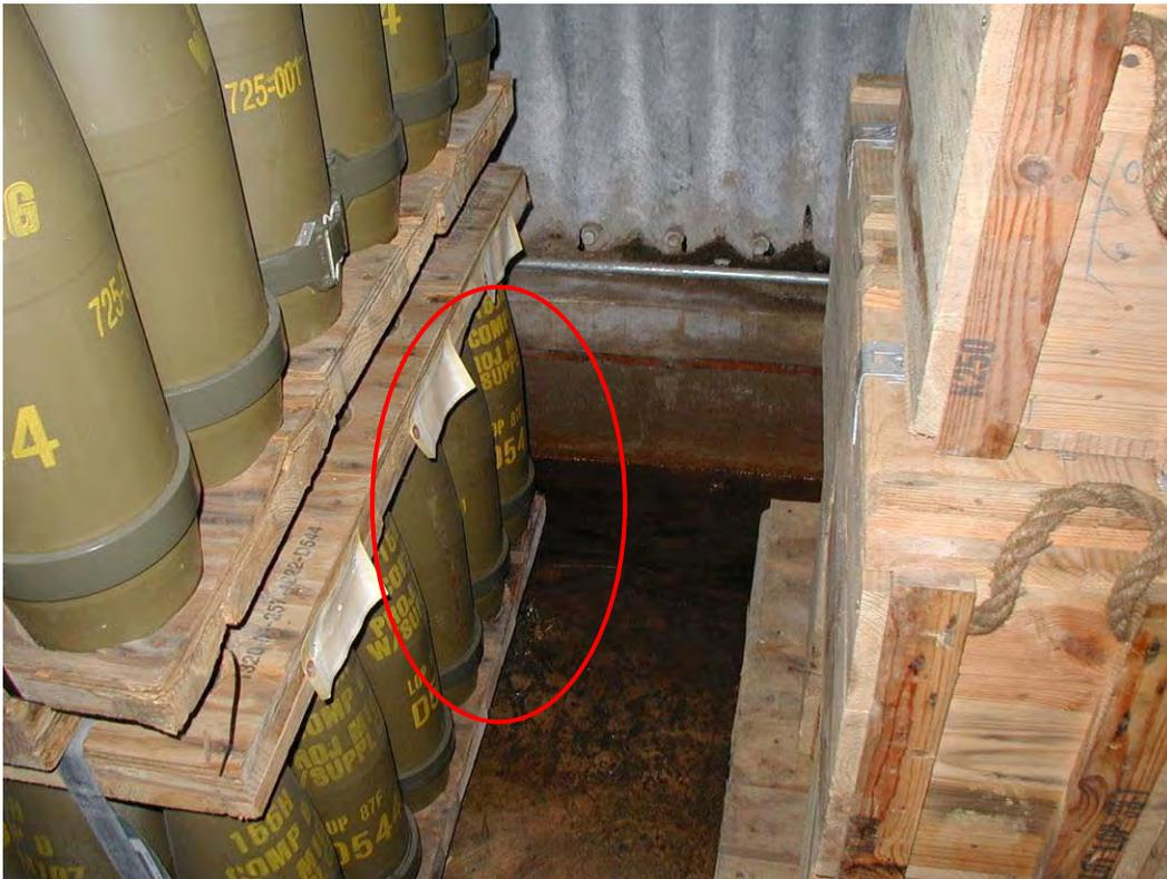
Figure 1: Corrosion on ammunition inside ammunition storage igloo.
