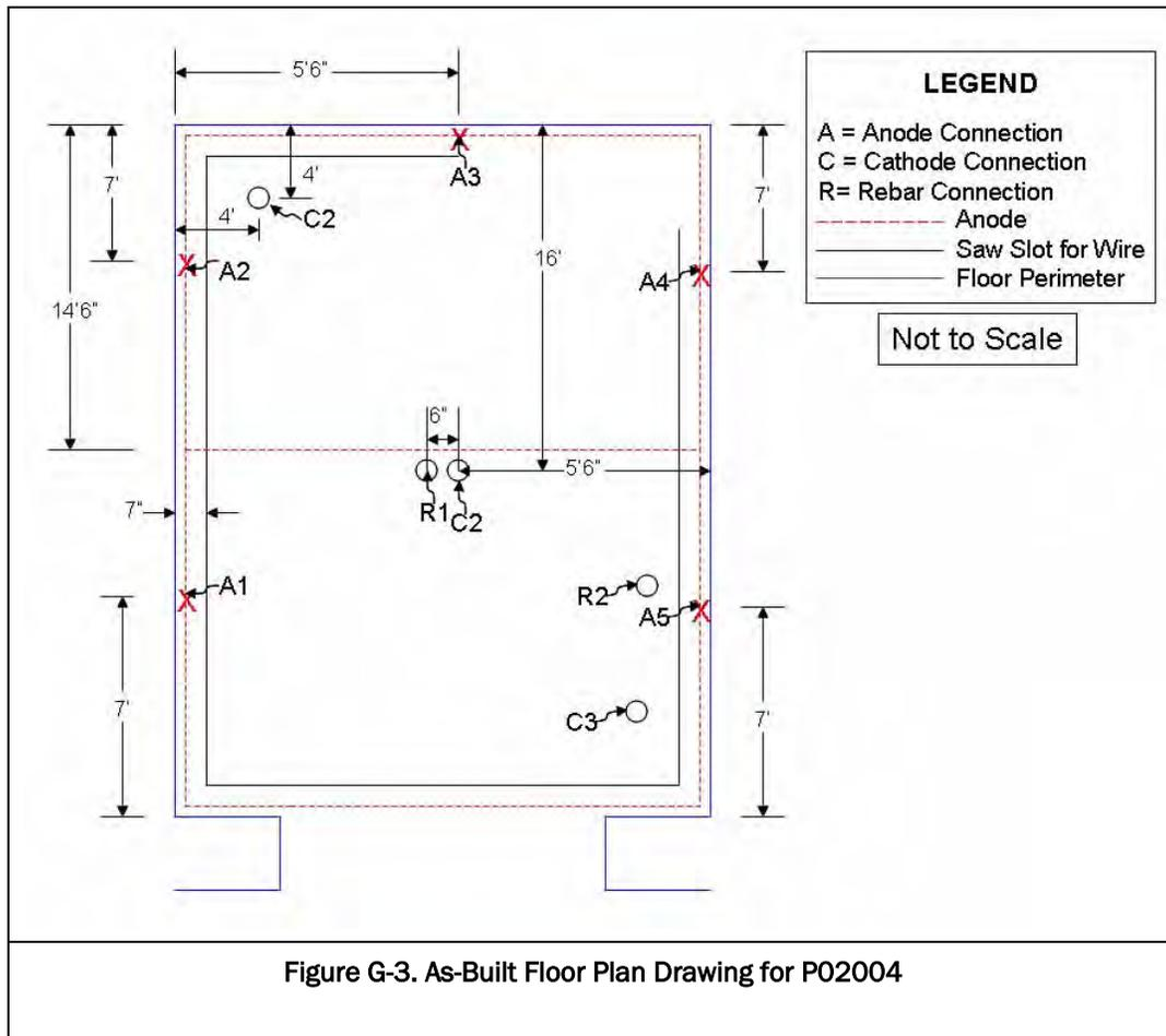
Figure G-3. As-Built Floor Plan Drawing for P02004
