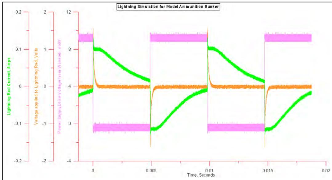
Figure C-11. Source signal for simulated lightning measurements on ECM model.
