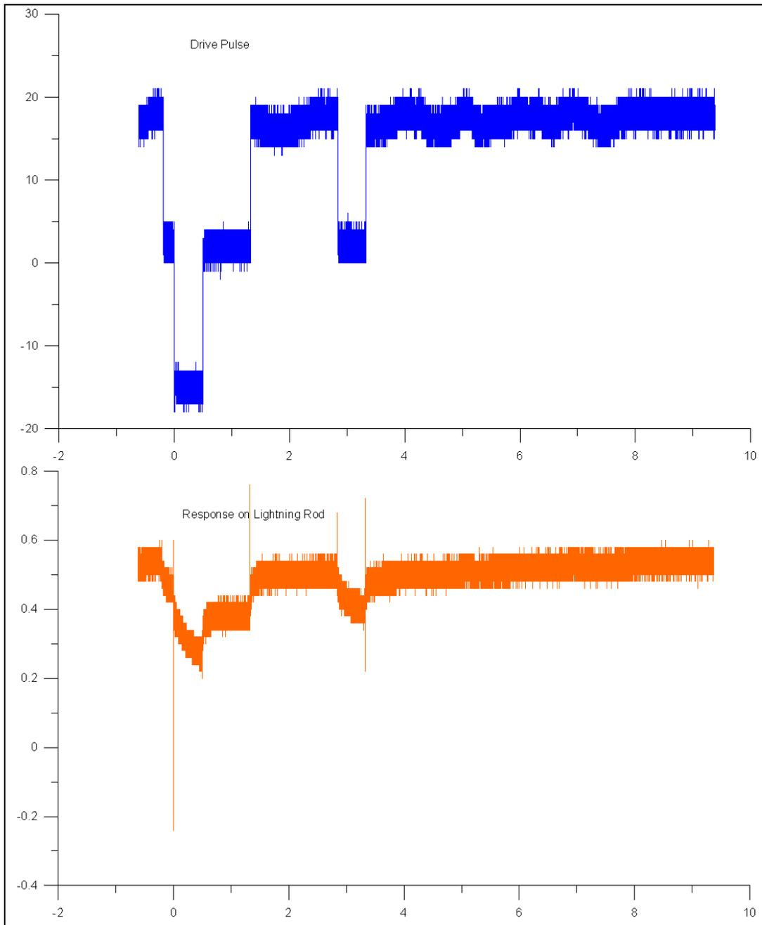
Figure C-12. EOP circuit current coupling to grounding system.
