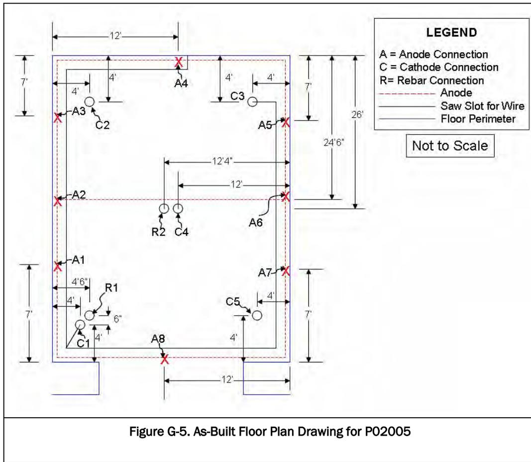
Figure G-5. As-Built Floor Plan Drawing for P02005
