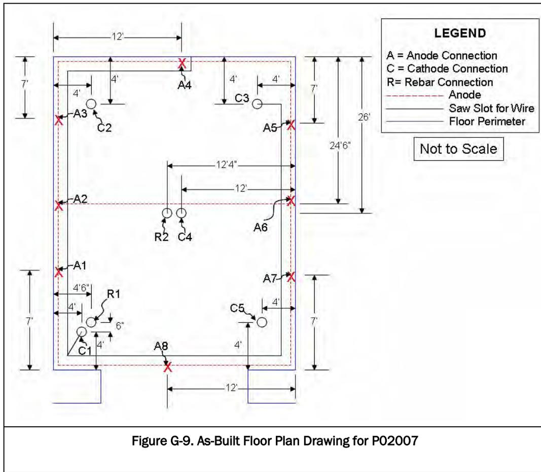
Figure G-9. As-Built Floor Plan Drawing for P02007
