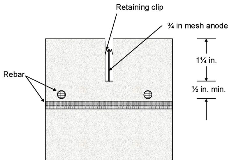
*NOTES: Mesh 3/4 in. wide and .05 in. thick expanded metal
