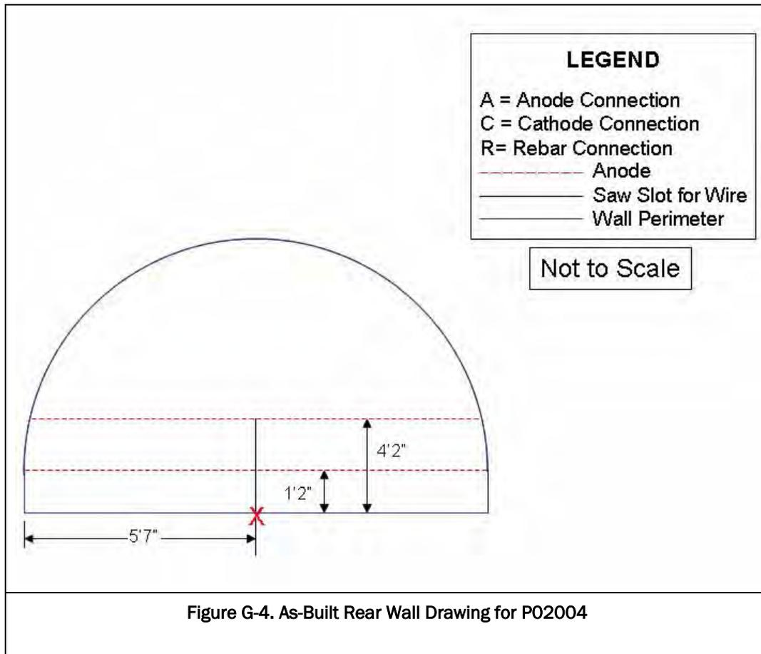
Figure G-4. As-Built Rear Wall Drawing for P02004
