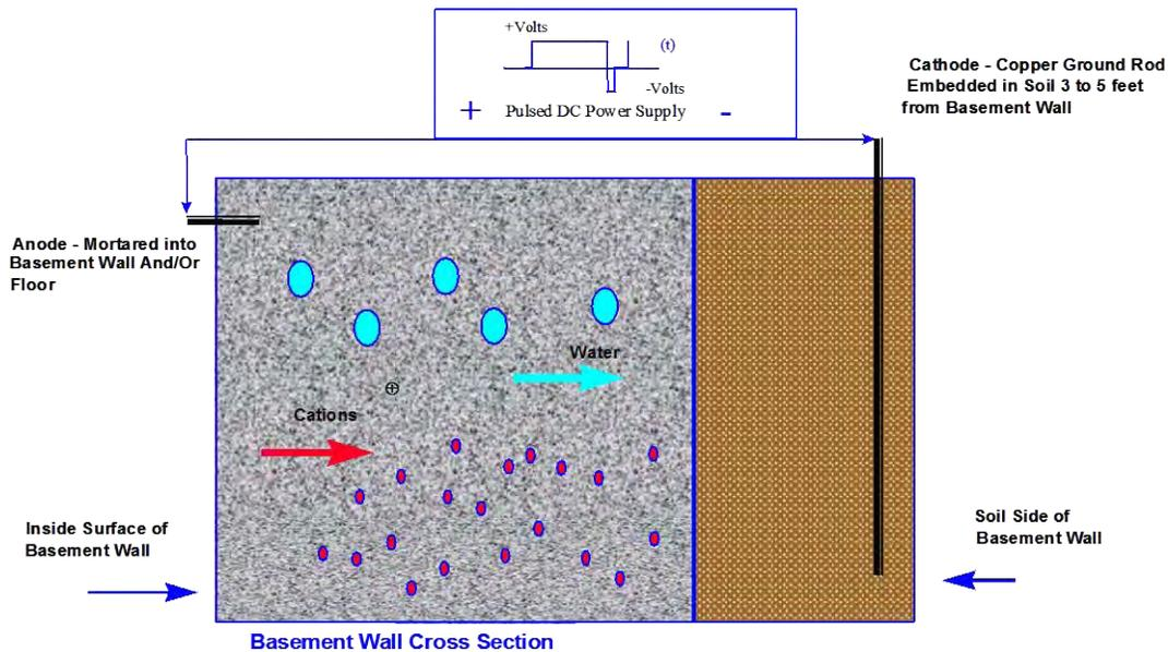
Figure 2: Schematic diagram of the Electro-Osmotic Pulse system.
